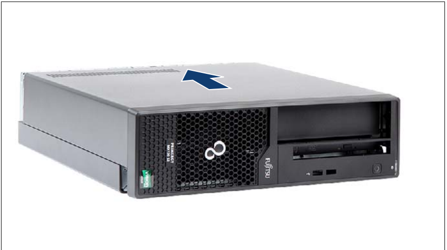
Figure 10: Closing the server cover
